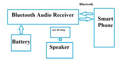
Bluetooth v2.0+edir, support a2dp Battery – Droid Incredible Phone Loudspeaker – Droid Incredible OP Amp – to be determined
