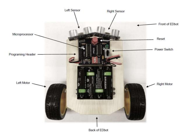
EDbot uses PIC18F1220 as the microcontroller with two independent DC motors and two independent distance sensors (HC-SR04) which make EDbot a highly flexible robotic platform. EDbot V7.0 schematic follows:
