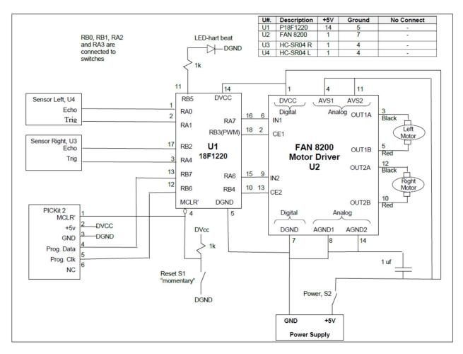
EDbot has specific assignment for all the PICmicro I/O Pins as follows:
