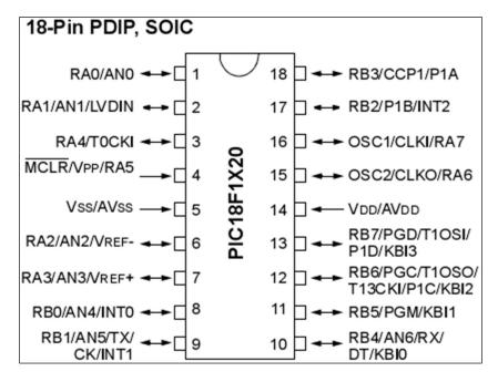
Each pin can be configured to perform a variety of functions, for example Pin 8 may be an I/O port (RB0), I/O port (AN4), external Interrupt 0 (INT0). This type of multi-use is common in microcontroller with high level of functionality but it is less common in general purpose microprocessors.
