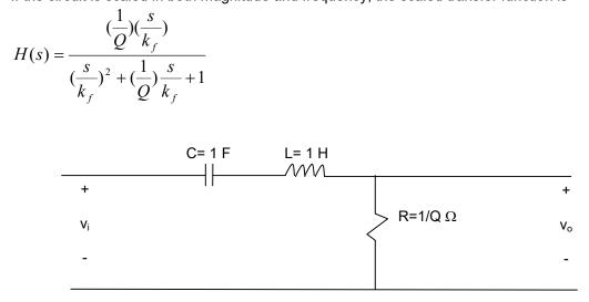
a) Specify the component values for the above prototype passive bandpass filter if the quality factor of the filter is 60.
