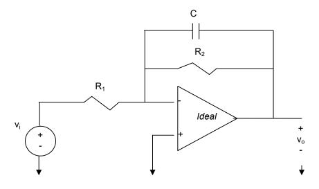
a) Design a low pass filter with a passband gain of 40 dB and a cutoff frequency of 5 kHz. Assume only a 0.5 uF capacitor is available.
