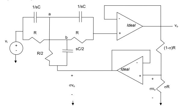
a) design a narrow-band bandreject filter having a center frequency of 1 kHz and a quality factor of 20. Base the design on C=15 nF.
