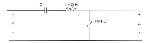
a) What is the value of C in the prototype filter circuit?
