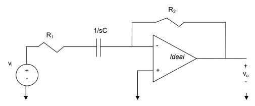
a) Design a high pass filter with a cutoff frequency of 25 kHz and a passband gain of 60 dB. Use only a 2.5 pF capacitor in the design.
