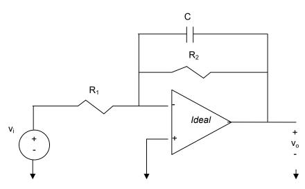
a) Design a low pass filter with a passband gain of 10 dB and a cutoff frequency of 1 kHz. Assume a 750 nF capacitor is available.
