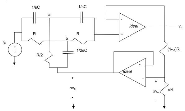
a) design a narrow-band bandreject filter having a center frequency of 5 kHz and a quality factor of 20. Use only C=10 nF in your design.
