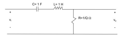
a) Specify the component values for the above prototype passive bandpass filter if the quality factor of the filter is 20.
