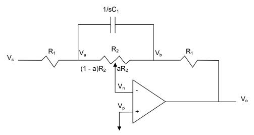
design a bass volume control circuit that has a maximum gain of 13.98 dB that drops off 3 dB at 50 Hz.
