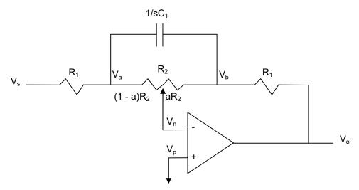
design a volume control circuit to give a maximum gain of 20 dB and a gain of 17 dB at a frequency of 40 Hz. Use an 11.1 k $\Omega$  resistor and a 100 k $\Omega$  potentiometer. Test your design by calculating the maximum gain at w=0 and the gain at w=1/R<sub>2</sub>C<sub>1</sub> using the selected values of R<sub>1</sub>, R<sub>2</sub>, and C<sub>1</sub>.
