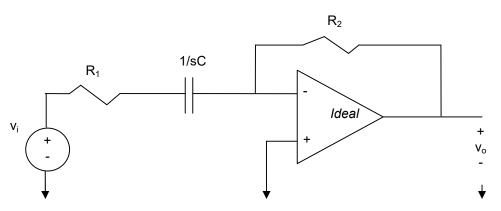
a) Design a high pass filter with a cutoff frequency of 8 kHz and a passband gain of 14 dB. Use a 3.9 nF capacitor in the design.
