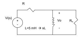
$$H_{loaded}(S) = \frac{Vo}{V_{1}} = \frac{Zeq}{R + Zeq} = \frac{\frac{1}{\frac{1}{sL} + \frac{1}{R_{o}}}}{R + \frac{1}{\frac{1}{sL} + \frac{1}{R_{o}}}} = \frac{(sL)(R)}{R(sL + R_{o}) + sLR_{o}} = \frac{jwLR}{RR_{o} + jwL(R + R_{o})}$$
