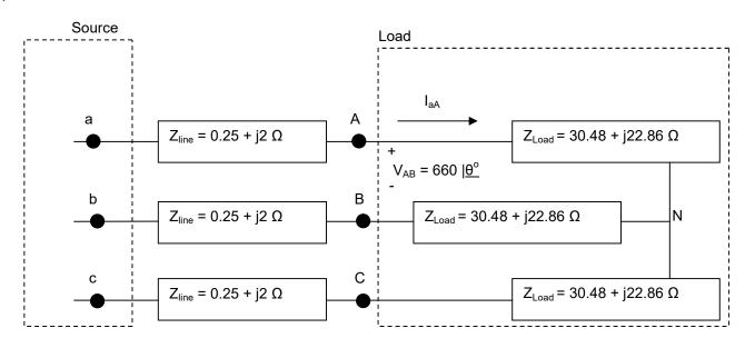
$$\mathbf{V}_{AN} = \frac{|V_{AB}|}{\sqrt{3}} |\underline{0 - 30^{\circ}} = \frac{660}{\sqrt{3}} |\underline{-30^{\circ}} = 381 |\underline{-30^{\circ}} V$$
