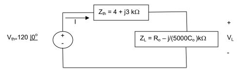
The condition for maximum power transfer is  $Z_{th} = Z_L^*$  therefore 4 + j3 = R<sub>o</sub> + j/5000C<sub>o</sub>  $\rightarrow$  Ro = 4 k $\Omega$ &
