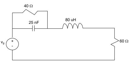
a) Find the average power, the reactive power and the apparent power supplied by the voltage source in the following circuit (Steady State).
