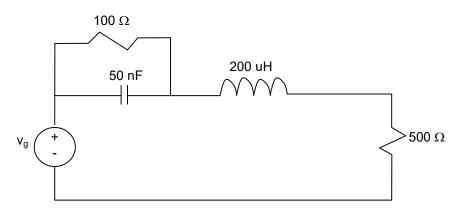
a) Find the average power, the reactive power and the apparent power supplied by the voltage source in the following circuit if.
