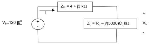
The condition for maximum power transfer is  $Z_{th} = Z_L^*$  therefore 4 + j3 = R<sub>o</sub> + j/5C<sub>o</sub>  $\rightarrow$  Ro = 4 k $\Omega$  & 1/(5000)C<sub>o</sub> = 3 k $\Omega$   $\rightarrow$  Co = 66.67 nf
