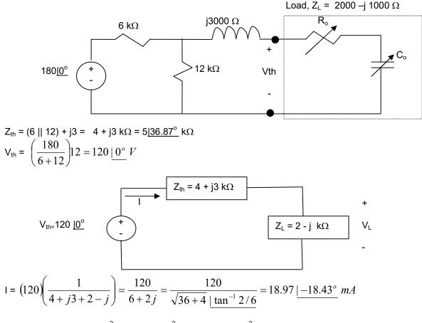
P = average power =  $|I_{eff}|^2 R_L = (1/2) |I_m|^2 R_L = (1/2)(18.97)^2 (2000) = 360 W$
