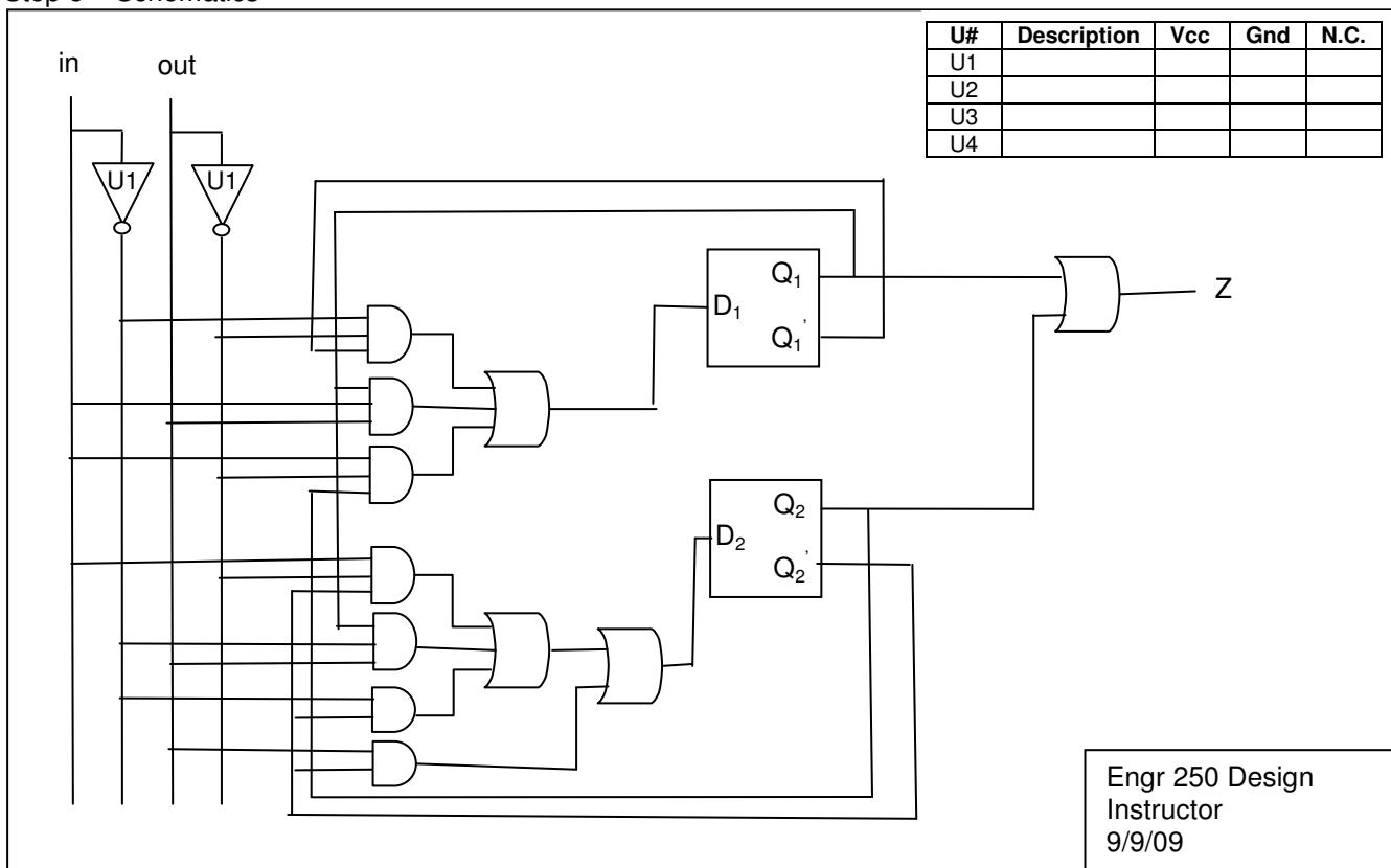
6U. Design a locking system with 8 keys (0 through 6 and \* keys). The system is locked normally and it unlocks only when the valid code sequence “\*236” has been entered. Entering any other sequence locks the system.
