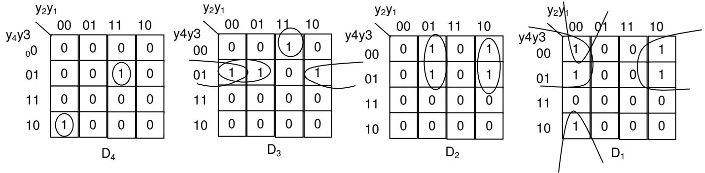
$$\begin{aligned}D_4 &= y_4y_3'y_2'y_1' + y_4'y_3y_2y_1 \\D_3 &= y_4'y_3'y_2y_1 + y_4'y_3y_2' + y_4'y_3y_1' \\D_2 &= y_4'y_2'y_1 + y_4'y_2y_1' \\D_1 &= y_4'y_1' + y_3'y_2'y_1'\end{aligned}$$
