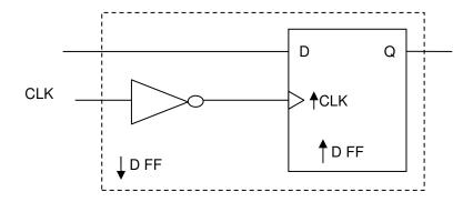
4U. Show how a positive-edge-triggered D flip-flop and other logic gates can be used to design a positive-edge T flip-flop.
