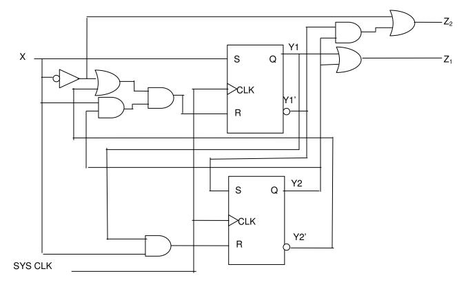
8S. Obtain the state diagram for the circuit shown below. What is the mod of the counter? Is this counter useful? Change only the value being loaded at the inputs to obtain a mod 9 counter. What value must be loaded to do this?
