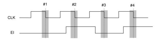
3U. Draw a clock signal CLK with five 0-to-1 timing events, a nonzero setup time,  $t_{su}$ , and a nonzero hold time,  $t_{h}$ . Also draw one excitation input signal EI that follows the sequence 10110 and meets the setup and hold time requirements. In the excitation input, the first bit in the sequence (1) occurs in time for the first clock timing event, the second bit in the sequence (0) occurs in time for the second clock timing event, and so forth.
