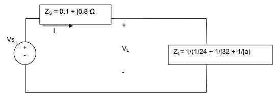
$\begin{aligned} |VL| &= |Vs| \; (Z_L/\; (Z_L + Z_S)) \\ \text{to Meet the condition} & \rightarrow (Z_L/\; (Z_L + Z_S)) = 1 \rightarrow \text{ since } Z_S \text{ is not 0 then } Z_L \text{ must be infinite} \end{aligned}$
