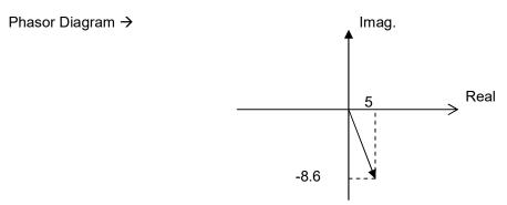
6U. Convert Steady State current i(t) = 30 cos (200t +  $\pi$ /6) to Phasor Domain and write out the equivalent current in Angular, Polar and Rectangular forms. Also draw the Phasor representation of this signal.
