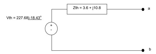
11U. Find the Thevenin equivalent circuit with respect to the terminals a, b for the circuit shown in the following figure.
