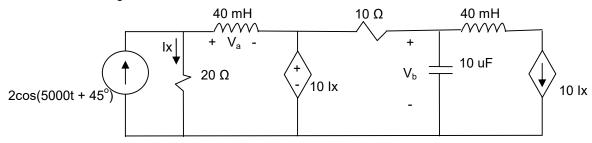
Find the relationship between  $V_a(t)$  and  $V_b(t)$  when the circuit is in steady state.
