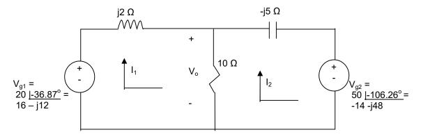
Step 3) Write the KVL equations for the two meshes:
