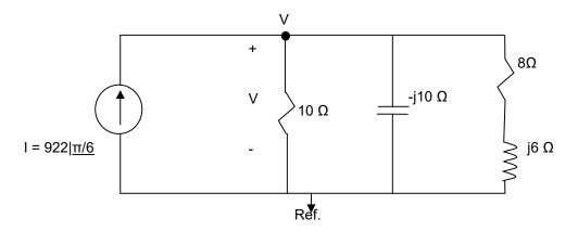
b) To find V, user Node-Voltage method and write the KCL equation for node V
