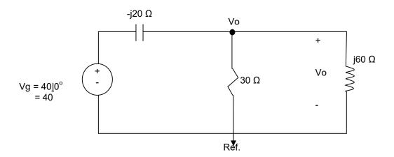
Step 2) Decide on Analysis method, Node Voltage is the simplest approach with 1 KCL equation So write the KCL for Node Vo
