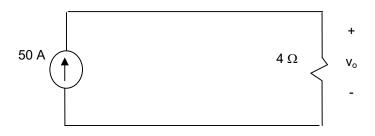
Simplified circuit  $\rightarrow$  V(o<sup>-</sup>)= 50\*4 = 200v Original circuit  $\rightarrow$  i<sub>0</sub>(o<sup>-</sup>) = 200 / 10 = 20 A
