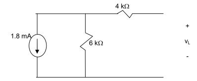
1.8 mA & parallel 6 k $\Omega$   $\rightarrow$  10.8 V and series 6 k $\Omega$
