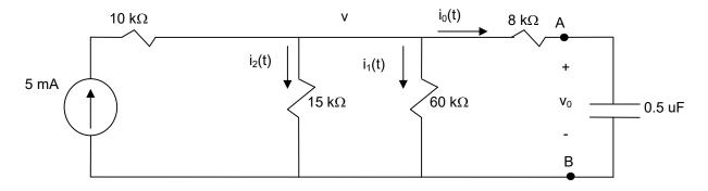
At  $t=0^+$ , Capacitor appears as a short  $\rightarrow$  Vo(0<sup>+</sup>)=0 V. KCL  $\rightarrow$  -5 + v/15 + v/60 + v/8 = 0  $\rightarrow$  25v = 5\*120  $\rightarrow$  v(0<sup>+</sup>) = 24 V  $\rightarrow$  i<sub>0</sub>(0<sup>+</sup>) = 3 mA
