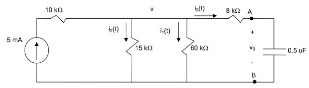
$$v(t) = 8,000 * i_0(t) + v_0(t) = 8 * 3e^{-100t} + 60 - 60e^{-100t} = 60 - 36e^{-100t}$$
