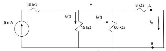
KCL  $\rightarrow$  -5 + v/15 + v/60 + v/8 = 0  $\rightarrow$  25v = 5\*120  $\rightarrow$  v(0 $^{+}$ ) = 24 V  $\rightarrow$  i<sub>sc</sub>= 3 mA
