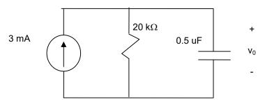
Apply the step response for RC circuit  $\rightarrow v(t) = I_s R + (V_0 - I_s R)e^{-t/RC}$  for  $t \ge 0$
