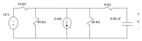
Use similar source transformation technique as used earlier will simplify the circuit into Norton equivalent.
