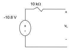
$$v_{L(0)} = 1.8 \text{ mA} * 6 \text{ K}\Omega = -10.8 \text{ V}$$
