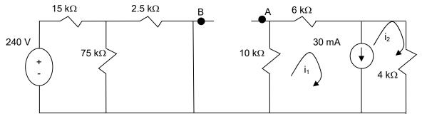
Choose B as the reference (v=0) and write the supper mesh current equation:
