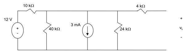
Use source transformation to simplify the circuit: 12v & series 10 k $\Omega$   $\rightarrow$  1.2 mA and parallel 10 k $\Omega$
