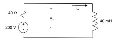
Apply the step response relationships  $i(t) = \frac{Vs}{R} + \left(I_0 - \frac{V_s}{R}\right)e^{-(R/L)t}$  for  $t \ge 0$
