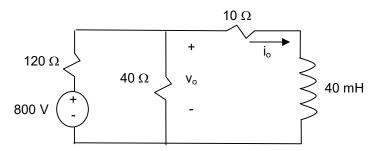
$$v_0(t) = 10i_0 + L\frac{di}{dt} = 10(5 + 15e^{-1000t}) + 0.04(-1000)(15e^{-1000t}) = 50 - 450e^{-1000t} \quad for \quad t \ge 0$$
