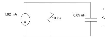
Apply the step response for RC circuit  $v(t) = I_s R + \left(V_0 - I_s R\right) e^{-t/RC}$  for  $t \ge 0$   $v_L(t) = -(0.00192)*(10,000) - \left(-10.8 - (-0.00192*10,000)\right) e^{-t/0.0005}$  for  $t \ge 0$   $v_L(t) = -19.2 + \left(+10.8 - 19.2\right) e^{-2000t}$  for  $t \ge 0$   $v_L(t) = -19.2 - 8.4 e^{-2000t}$  for  $t \ge 0$
