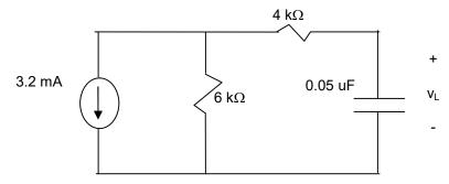
3.2 mA & parallel 6 k $\Omega$   $\rightarrow$  19.2 V and series 6 k $\Omega$  Another source transformation reduces the circuit to:
