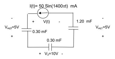
0.30 mF, 0.30 mF and 1.20 mF are in series  $\rightarrow$  Ceq4 = 0.13 mF with V = 10-5 +5 = 10 V
