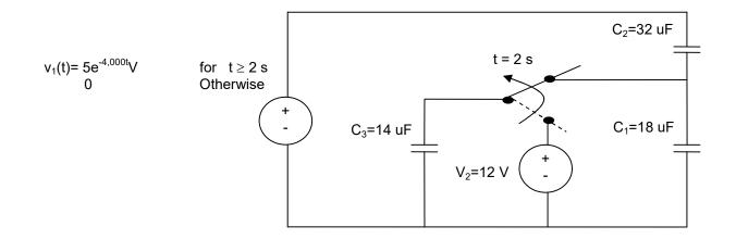
$$V_{C3}(2) = 12 \text{ V}, \quad V_{C2}(2) = 0 \text{ V}, \quad V_{C1}(2) = 0 \text{ V}$$
