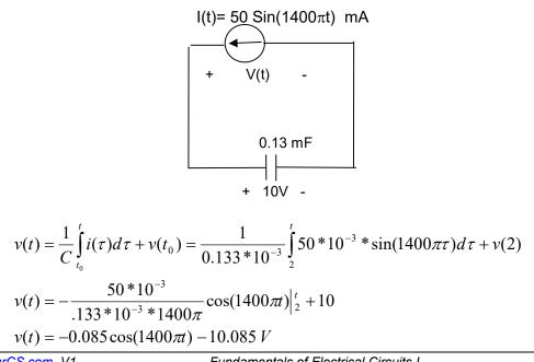
8U. In the following circuit, find the equation for voltage across the current source, v(t) for  $t \ge 5$  sec.
