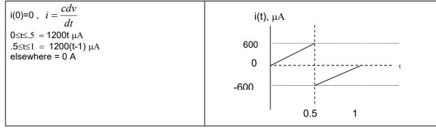
2U. A 10 uF capacitor is subjected to a voltage pulse having a duration of two seconds. The pulse is described by the following equations:
