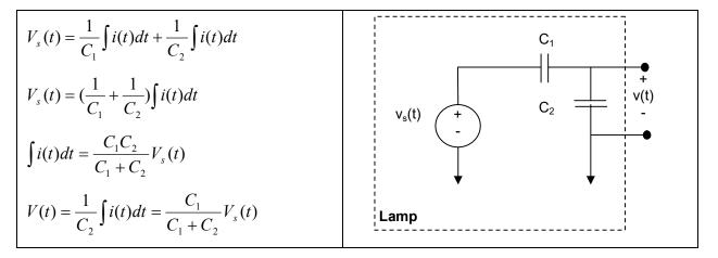
Using the above analysis result fot the circuit when no person touching, only 10 pF goes to ground. Therefore
