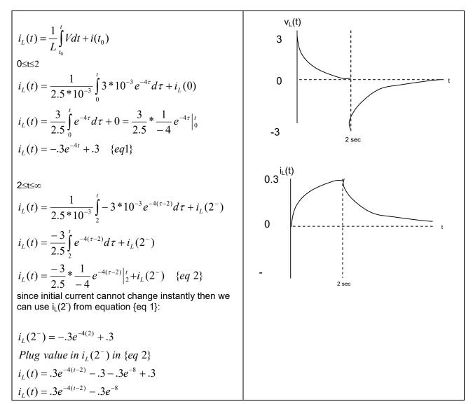
1U. The current in the 2.5 mH Inductor in the following figure is known to be 0A for t<0. The inductor voltage for  $t\geq 0$  is given by the expression:
