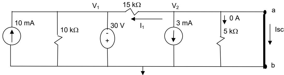
$$V_1 = -30 \text{ V}$$
