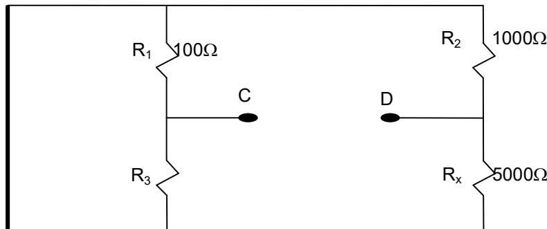
$$R_{CD\text{ eq}} = R_{th} = (100 \parallel R_3) + (1000 \parallel 5000) = 100R_3/(100+R_3) + 5000/6$$
