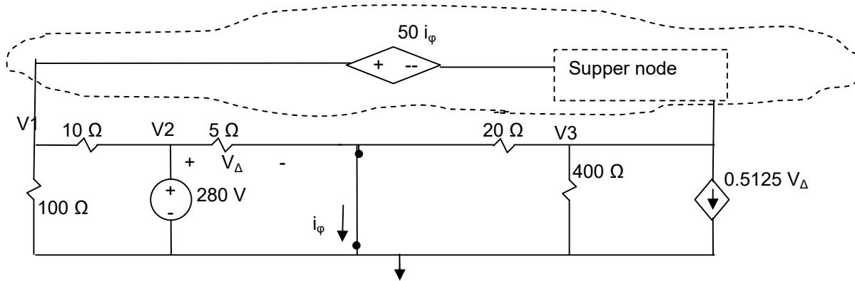
$$\text{KCL at } V_2 = 280 \text{ V} \rightarrow V_2 = V_\Delta = 280 \text{ V}$$
