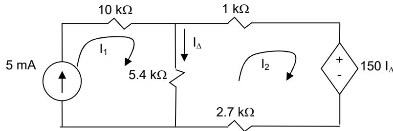
$$\text{We have } I_1 = 0.005 \text{ A} \quad & I_\Delta = I_1 - I_2$$
