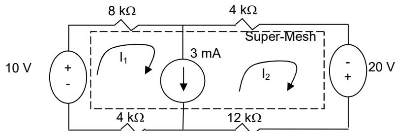
$$\text{Super-Mesh KVL} \rightarrow -10 + 8I_1 + 4I_2 - 20 + 12I_2 + 4I_1 = 0 \rightarrow 12I_1 + 16I_2 = 30$$
