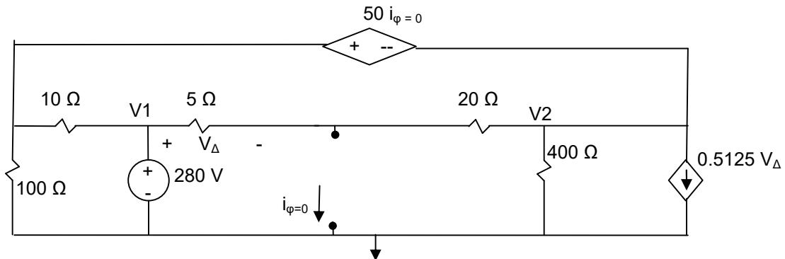
KCL at  $V_1=280$  V
