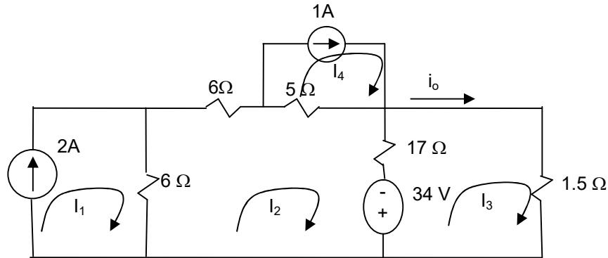
$$\text{KVL for Mesh #1} \rightarrow I_1 = 2 \text{ A}$$
