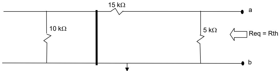
$$R_{th} = ((10 \parallel 0) + 15) \parallel 5 = 3.75 \text{ k}\Omega$$
