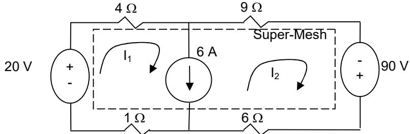
$$\text{Super-Mesh KVL} \rightarrow -20 + 4I_1 + 9I_2 - 90 + 6I_2 + I_1 = 0 \rightarrow 5I_1 + 15I_2 = 110$$
