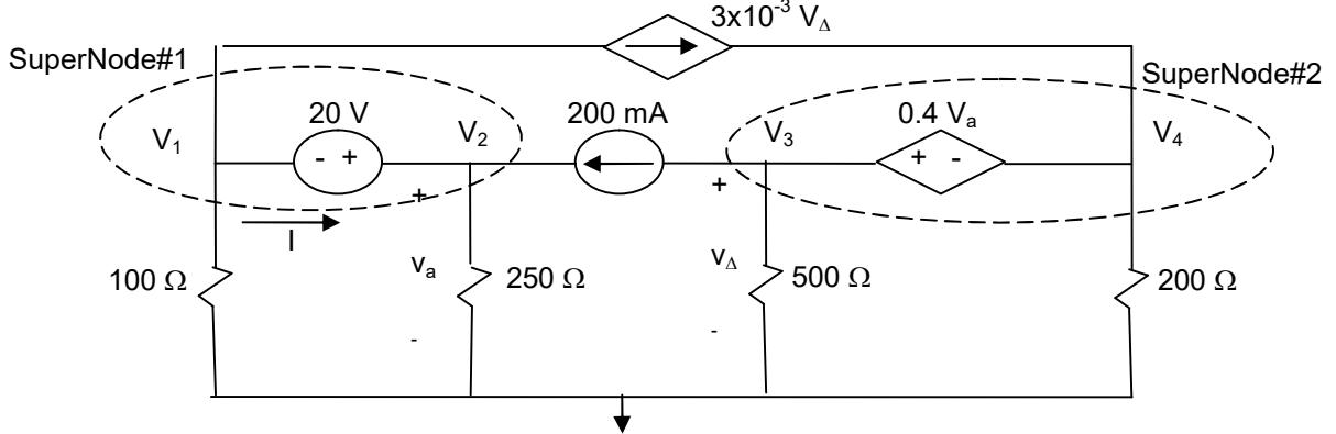
$$\text{Super Node #1 KCL} \rightarrow -0.2 + .003V_\Delta + V_1/100 + V_2/250 = 0$$
