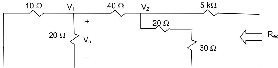
$$R_{eq} = (((10 \parallel 20) + 40) \parallel (20 + 30)) + 5000 = 5024.15 \text{ }\Omega$$
