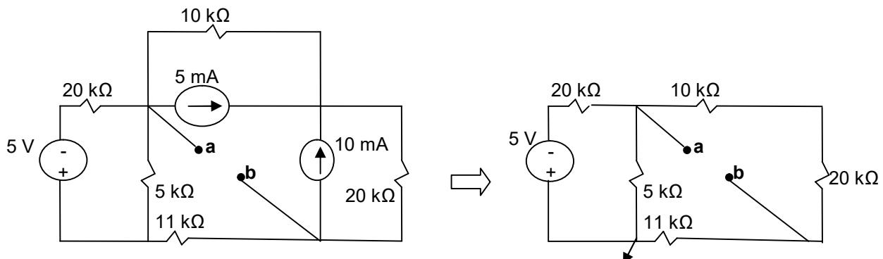
$$(V_a - (-5)) / 20 + (V_a - V_b) / 30 + V_a / 5 = 0 \quad 17 V_a - 2 V_b = -15$$
