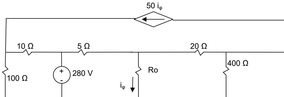
For the above circuit, find the Thevenin equivalent with respect to terminals of  $R_o$ .
