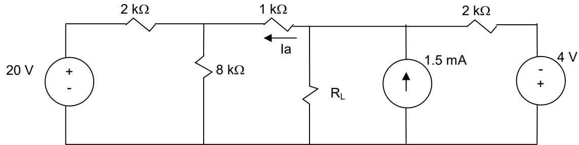
*Hint: Find  $R_{th}$  with respect to  $R_L$  terminals First.*
