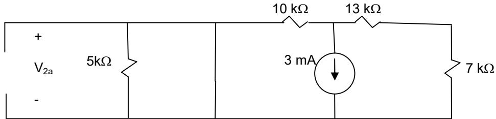
$$R_{eq} = 0 \text{ k}\Omega \rightarrow V_{2a} = 0 \text{ V}$$
