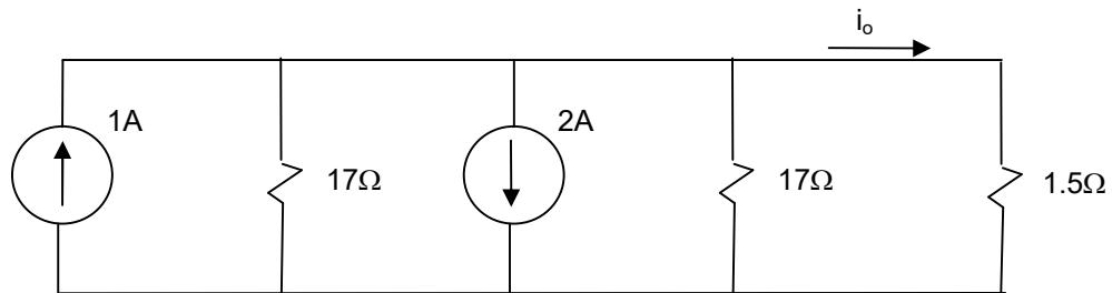
Simplify by adding current source and Req for  $17 \parallel 17 = 8.5 \Omega$
