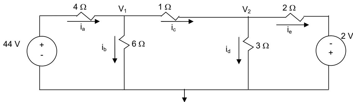
a) Three essential nodes so we can write 2 Node-Voltage Equations:
