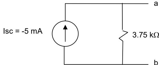
10U. Find the Norton equivalent with respect to the terminals a,b in the following circuit.
