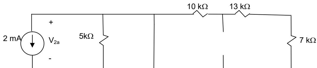
$$R_{eq} = 0 \text{ k}\Omega \rightarrow V_{2a} = 0 \text{ V}$$
