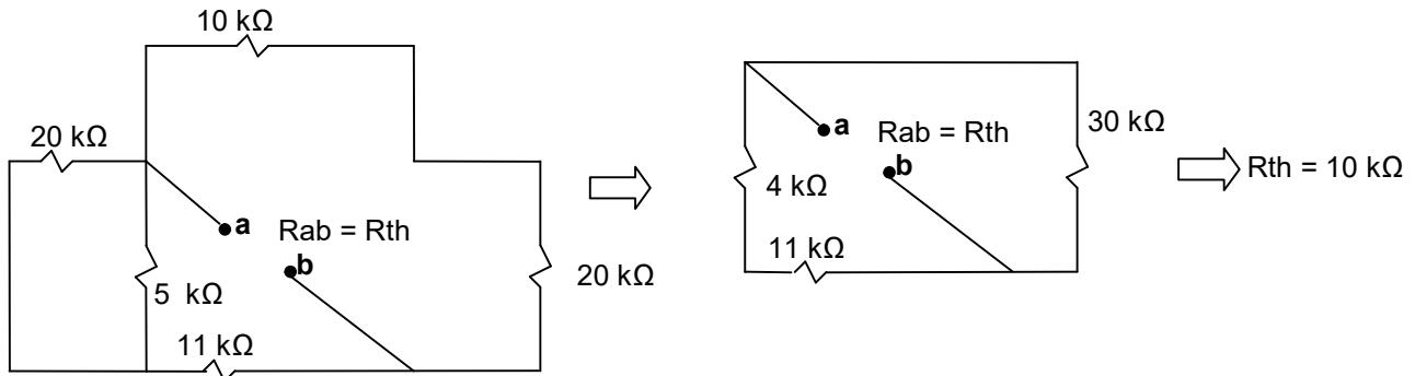
Now find Open circuit voltage ( $V_{th}$ ):
