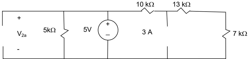
$$V_{2a} = + 5 \text{ V}$$
