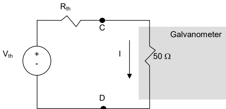
$$I = V_{th} / (R_{th} + 50) = (5 \cdot R_3 / (R_3 + 100) - 25/6) / ((5000/6 + 100R_3/(100+R_3) + 50) \text{ when } R_3 = 501)$$
