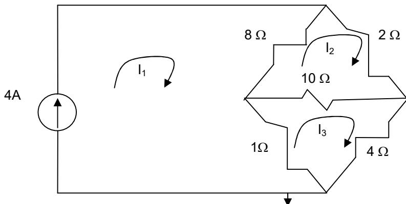
$$\text{KVL for Mesh\#1} \rightarrow I_1 = 4 \text{ A}$$
