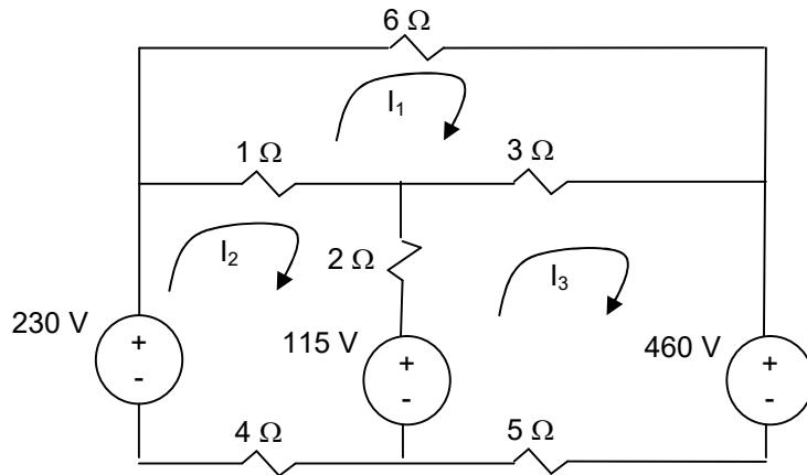
$$\text{Loop #1 KVL} \rightarrow 6I_1 + 3(I_1 - I_3) + (I_1 - I_2) = 0$$
