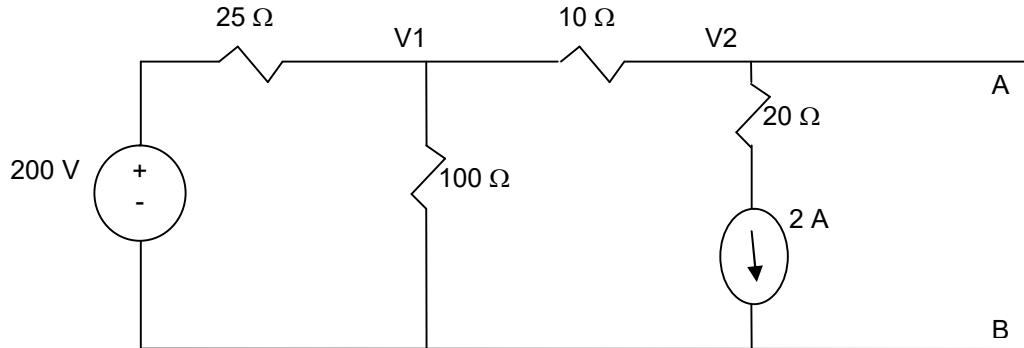
$$\text{KCL at } V_1 \rightarrow (V_1 - 200)/25 + V_1/100 + (V_1 - V_2)/10 = 0$$
