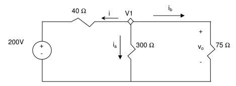
KCL at V1  $\rightarrow$  (V1 - 200)/40 + (V1 - 0)/300 + (V1 - 0)/75 = 0 Simplify equation 1  $\rightarrow$ 25V1 = 3000  $\rightarrow$  V1 = 120 V
