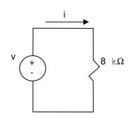
1U. The terminal voltage and terminal current were measured on the device shown below. The values of v and I are given in the table below. Use the values in the following table to construct a circuit model for the device consisting of a single resistor.
