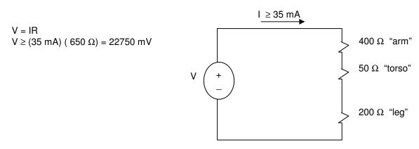
8Sd. A person accidentally grabs conductors connected to each end of a dc voltage source, one in each arm. Assuming each arm has a resistance of  $400\Omega$ , Calculate the minimum voltage from the dc voltage source required to shock the person (35 mA is sufficient to shock). Draw the equivalent circuit diagram.
