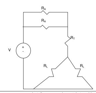
7U. Suppose the power company installs some equipment that could provide a 250V shock to a human being. Is the current that results dangerous enough to warrant posting a warning sign and take other precautions to prevent such a shock?
