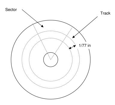
There are 77 track on one disk side, which would account for 700k bytes. Each track is 1/77 in. apart from center to center.
