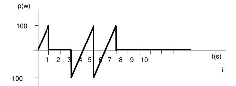
b) Calculate the energy delivered to the circuit element at t=1, 6, and 10 s. To find the answer simply sum the area under the curve to the time stated:
