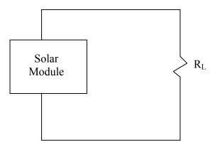
Show the steps used to calculate the value of  $R_L$  Also document the process used to show that the calculated  $R_L$  value does or does not receive maximum load power. Explain the reasons for any variances you observe.
